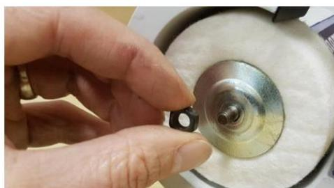
Carefully slide the mop onto the shaft, replace the plate flange, the nut and tighten against the rotation of the mop.
