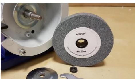
Remove the plate flange and carefully remove the stone.
