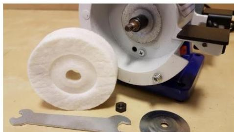
Remove the plate flange and carefully remove the mop.
