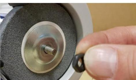
Inspect the new stone for cracks and damage to either the front face or the edges before fitting.
