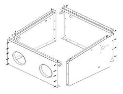
4.2 Use M6x12 bolts to connect cabinet,funnel and feet. Please note the bolts must insert from cabinet and nut from bottom
