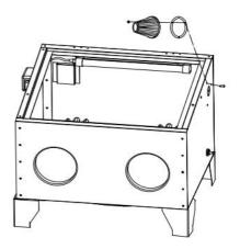
4.6 Connect the hinges in the top door with ST4\*8 screw to the cabinet.
