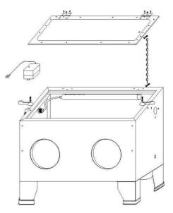
4.7 Assemble the gloves to the front plate by clamps  $\Phi$  120- $\Phi$  150.
