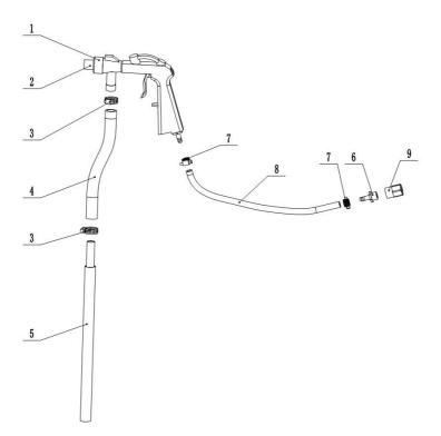
1. Connect sand hose (No.4) with gun(No.2), clamp (No.3)it.Connect sand pipe (No.5) into sand hose and clamp it.
