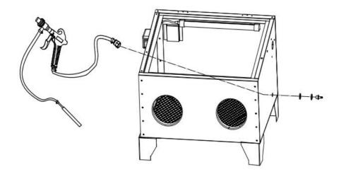
Install sandblasting gun, rubber and metal washer to the inner thread connector of right cabinet plate.
