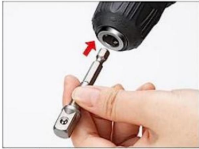
Step 1: Install the connecting rod on the electric drill bit and tighten it
