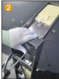
2 Use 2 M4 screws to secure the main fixed plate and top spray
