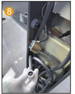
8 Spray socket with hexagonal nut handle. Fix the 4-point rubber on the panel and spray it by hand inside the seat joint
