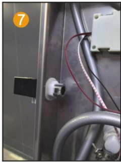
7 Spray socket with hexagonal nut handle fixed on the panel
