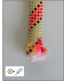
• Damaged rope end
