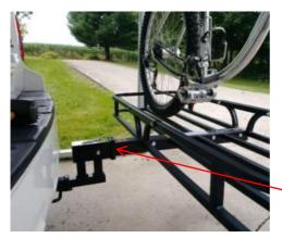
All accessories (bike rack, cargo carrier, etc.) must be secured to the top receiver (with collar) with a steel hitch pin and B-Shaped safety clip. Make sure safety clips are always fully engaged.
