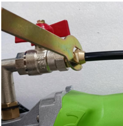
3. Install water pipe joints, Lock with a wrench.
