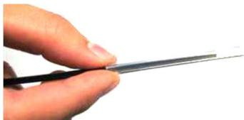
Put the fiber through the splicing tube so to protect fusion point after splicing. Make sure there is no impurity inside the tube and keep the tube parallel with the fiber.
