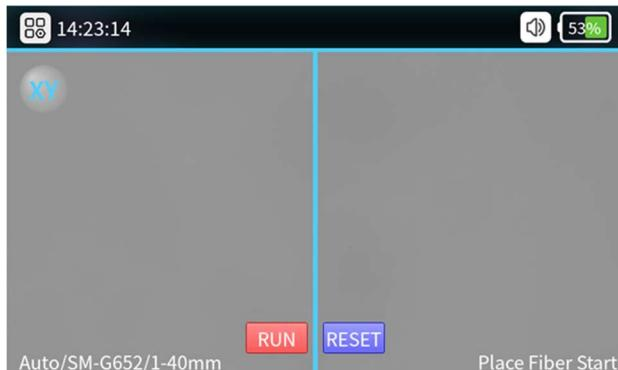
Optical fiber observation interface: Short push the power switch then the indicator on the operation panel will turn to red and the buzzer will be sounds like “Di Di”. All motors will return back to their initial positions and the fiber observation interface shows.
