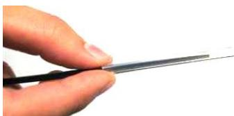
Put the fiber through the splicing tube so to protect fusion point after splicing. Make sure there is no impurity inside <sup>19</sup> the tube and keep the tube parallel with the fiber.
