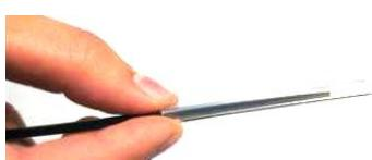
Put the fiber through the splicing tube so to protect fusion point after splicing.
