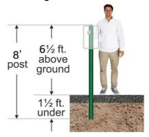
3. Try Two Posts Instead: Professionals often use two overlapping 6' posts. This gives the signs plenty of headroom (thereby avoiding needless pedestrian accidents). Installing two sign, surprisingly, can be quite easy. See the next photo. Generally, we recommend from 6" to 12" of overlap between the two posts. It is not possible to overlap two medium weight 1.12 lbs posts.
