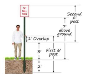
4. Pounding in the Post: Posts are generally pounded into the ground (unless a sand-filled sleeve is used). For all but the shortest posts, we recommend using the bed of a pickup truck as your platform.
