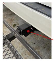
All accessories (bike rack, cargo carrier, etc.) must be secured to the top receiver (with collar) with a steel hitch pin and B-Shaped safety clip. Make sure safety clips are always fully engaged.
