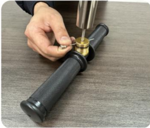
2. Remove the handle fixing pin.
