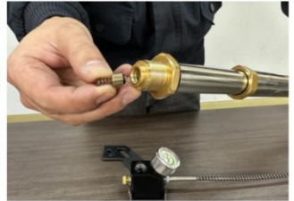
12. Install the check valve.
