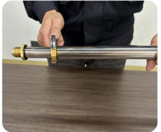
3. Loose the primary piston and remove the primary tube.
