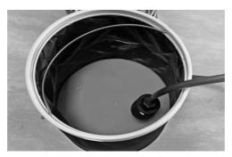
Step 5: Install the foam pot: Insert the foam pot into the barrel and rotate the clamp as shown.
