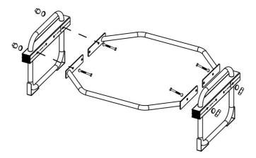
2.2. Thread in and tighten the left and right wall hanging screws according to the requirements in the diagram in sequence .
