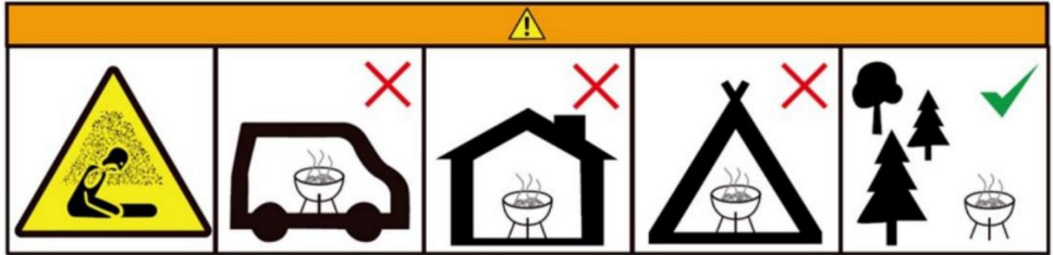
Carbon Monoxide Poisoning Hazard
