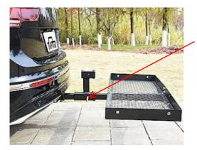
All accessories (bike rack, cargo carrier, etc.) must be secured to the top receiver (with collar) with a steel hitch pin and B-Shaped safety clip. Make sure safety clips are always fully engaged.
