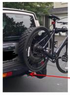
All accessories (bike rack, cargo carrier, etc.) must be secured to the top receiver (with collar) with a steel hitch pin and B-Shaped safety clip. Make sure safety clips are always fully engaged.
