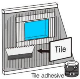
6. Remove the protective film of the tape, apply a uninterrupted bead of silicon sealant from the inside corner of the niche to the edge Ensure
