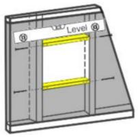
4. Glue waterproofing membrane inside to seal the whole cave and extend 6inch to four sides of surrounding wall. **Create watertight seal cave is very important.**
