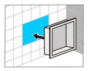
8. Tape the flanges with wall to hold the niche in place until the sealant cured.
