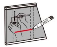
2. Trace the cut line with pencil, above the center line, cut out a cave on the wall board along the traced line. Be sure the top and bottom lines are level.
