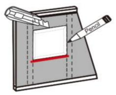
3. Level and fasten the surrounding framing to adjacent vertical studs make the dimension matches the niche flange.
