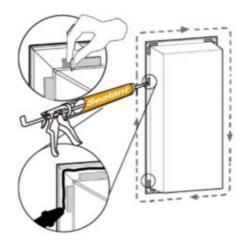
7. Insert the niche fixture into the cave . Press the flange tightly and ensure the niche plumb and level . Wipe off the excess sealant along the perimeter edges.
