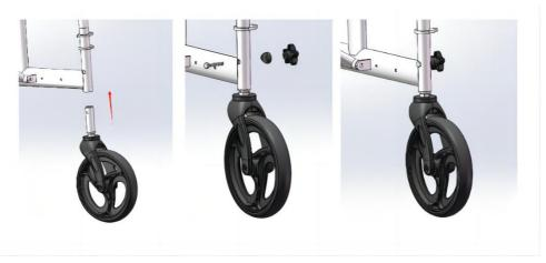
1.As shown in the figure: Place the front wheel into the main frame pipe bend, align it with the hole position, and lock it with screws and knobs.
