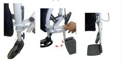
7. As shown in the figure: Install the right foot pedal assembly into the pin on the right side of the main frame, rotate it to the left to fix the foot pedal assembly.
