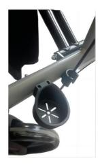
9. As shown in the figure: Install the crutch holder into the crutch holder.
