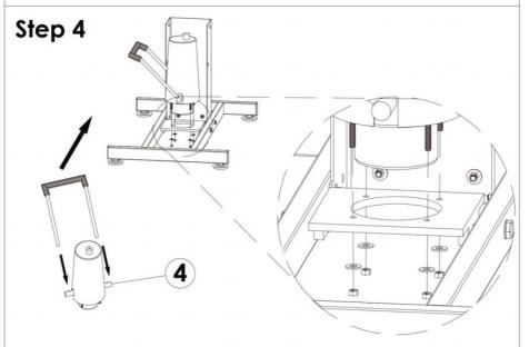
Please remove the foam wrapped on the hydraulic pump before installation
