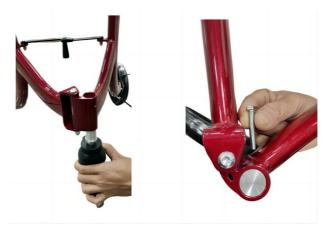
4.As shown in the figure: Insert the front wheel into the main frame, align the screw hole of the front wheel lever with the hole of the main frame, and thread the hexagonal screw through.
