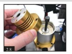
9. Take off the column metal part, clean dirt inside and check the low-pressure o-rings if any damaged. You can add a little silicone or motor oil on piston o-ring.
