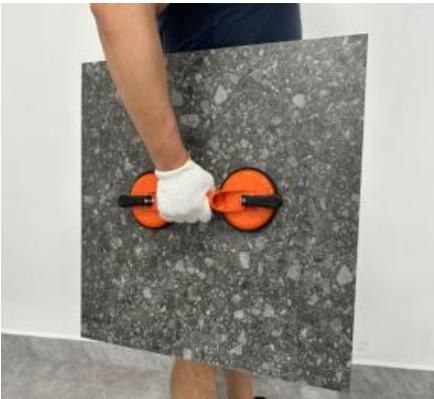
4. After moving the item, pull the handle back to its original position, allowing the suction pad to return to its flat state and release the vacuum pressure, thus completing one lifting operation. If the suction cup remains attached to the item and cannot be removed, you can slightly lift the edge of the suction pad with your finger to let air into the vacuum cavity and separate the two.
