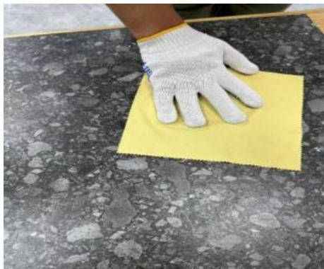
2. The surface of the item to be lifted must be wiped clean.
