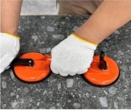
3. Place the suction pad flat against the item and press firmly on the item's surface while simultaneously pulling down the plastic handle. The suction pad will be lifted and deformed, creating a cavity with a considerable vacuum between the suction pad and the item. The atmospheric pressure causes the suction cup to hold the item firmly. At this point, the item can be lifted and moved by hand.
