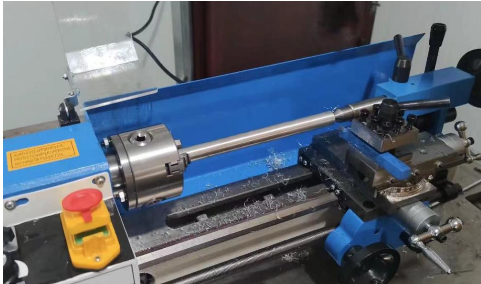
Fig 6 Workpiece Holding And Drilling
