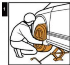
Jack up the car and de-mount the tire.
