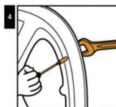
Tighten the valve by wrench and screw it ( Torque value must be \geq 4\text{Nm} )
