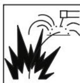
**Fire hazard.** Welding/cutting on closed containers, such as tanks, drums, or pipes, can cause them to explode. Flying sparks from the welding/cutting arc, hot work piece, and hot equipment can cause fires and burns. Accidental contact of electrode to metal objects can cause sparks, explosion, overheating, or fire.
