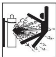
**Gas Cylinders.** Shielding gas cylinders contain gas under high pressure. If damaged, a cylinder can explode. Because gas cylinders are normally part of the welding/cutting process, be sure to treat them carefully. CYLINDERS can explode if damaged.
