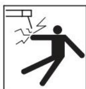
**Electric shock: It can kill.** Touching live electrical parts can cause fatal shocks or severe burns. The electrode and work circuit is electrically live whenever the output is on. The input power circuit and internal machine circuits are also live when power is on. In MIG/MAG welding, the wire, drive rollers, wire feed housing, and all metal parts touching the welding wire are electrically live. Incorrectly installed or improperly grounded equipment is dangerous.
