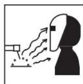
**Arc rays:** harmful to people's eyes and skin. Arc rays from the welding/cutting process produce intense visible and invisible ultraviolet and infrared rays that can burn eyes and skin. Always wear a welding helmet with correct shade of filter lens and suitable protective clothing including welding gloves whilst the welding/cutting operation is performed.
